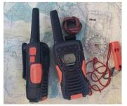
We've also used the rugged AM1055 FLT radios from Cobra featuring a floating & waterproof (IPX7) design.
